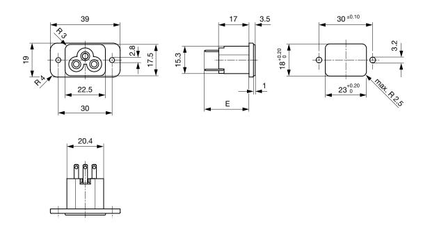
E: Solder terminals short: 18.9 mm E: Solder terminals long: 22.6 mm
